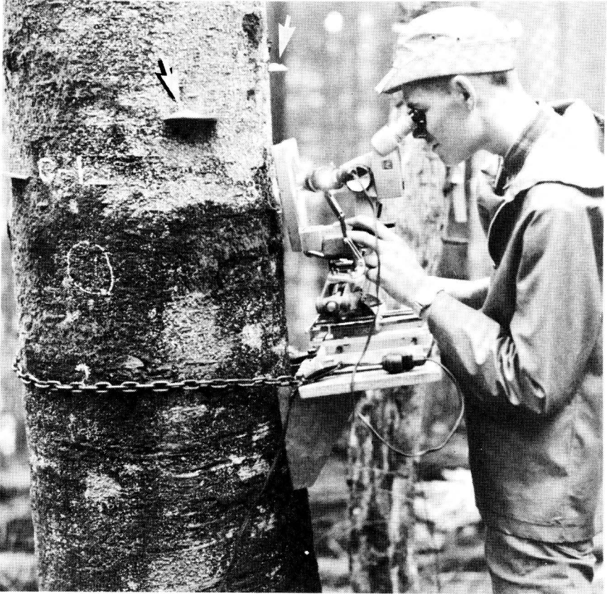
Fig. 1. Examination of bole with microscope mounted on scissor jack on portable platform and showing tanglefoot drop cards (arrows) in position on the bole.
