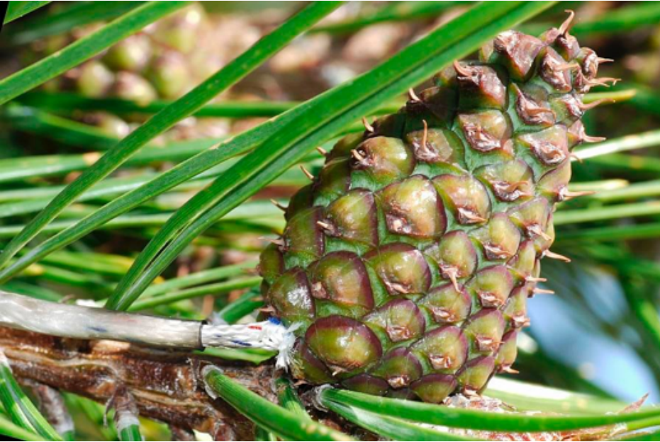
Figure 1. Thermocouple wire inserted into a 1-mm hole drilled into the seed-bearing portion of a lodgepole pine cone.
